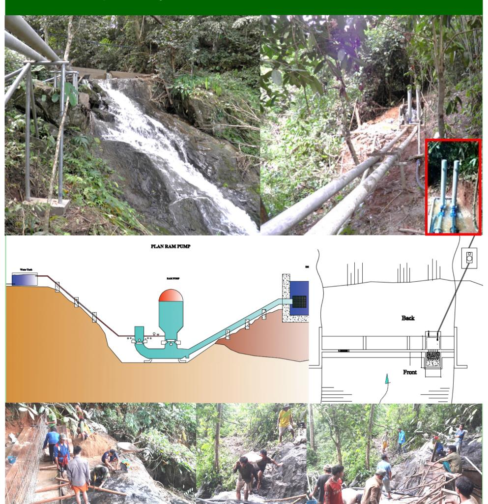
**Innovation**: Hydraulic Ram Pump use the force of gravity to pump up the water, without using any electricity and gasoline – thus keeping the costs of operations and maintenance at a minimum.
